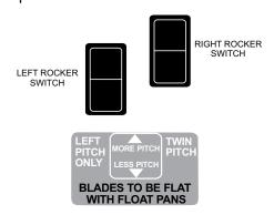
Figure 17. Blade Pitch Rocker Switches
